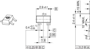
1) Lead width can be 0.6 max. in dambar area
